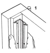
Close door and bend fixing strip to an 'L' shape you will then have 2 sections one longer than the other, hold in the corner of the frame and door as shown being sure to keep the wider section on the door side.
