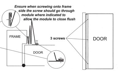
When screwing to the door side, ensure the 3 screws are inserted into the clip and module. On the frame side, it is screwed only through the module (as shown in diagram), as this will ensure the strip will lay flat against the frame when it is closed.
