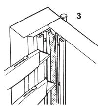
With Stanley knife separate strips at corner and remove spacer from door (if strip is not removed, the door will not close).
