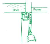
Roll the MK1B over the hinges and butt the T shape to hinges on frame side. Align with L shape top and bottom. Secure with TEK self tapping screws and remove cellophane protective membrane. You are now findersafe
