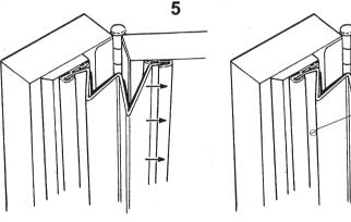
Insert 3 inch panel of fingersafe in door fixing strip.
