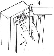
Open the door 90 degrees and align the 1 inch side of the pleated panel to the frame side of the fixing strip. Then snap into position, top to bottom.
