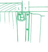
MK1B must be cut square aligned with top and bottom of door
